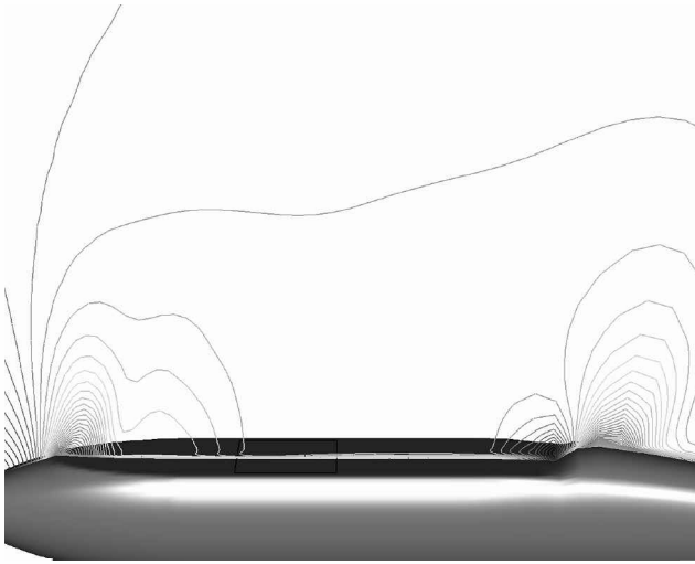
Fig. 8 Pod at Mach number M_\infty = 0.9 , density distribution.
