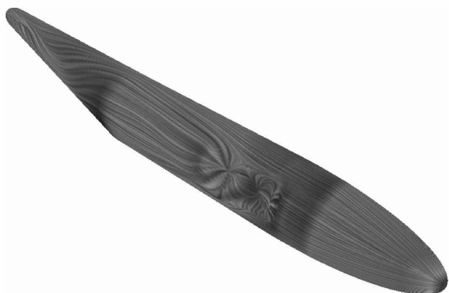
Fig. 6 Original pod at Mach number M_\infty = 1.2 , skin-friction lines shaded by values of local pressure.
